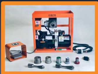
Bench-top 1690 and 1691 portable expander with hands-free foot pedal operation
