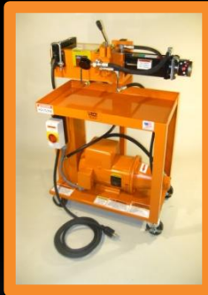
Model 1673: Portable Expander- Swager for versatile end finishing
