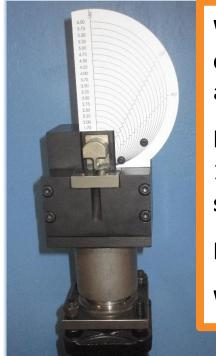
Works with any 3.5" Huth expanding cylinder on benders, benchtop expanders and other portable swagers and expanders.
