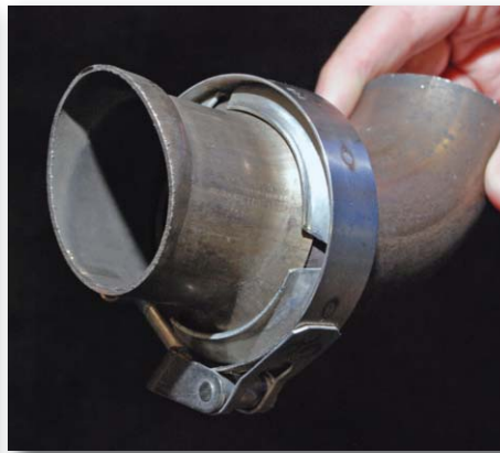
Huth V-Band Segment Set Tooling and a piece of formed tubing.
